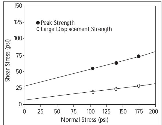
**Figure 3.** ASTM D-6243, Direct Shear Test data for GCL.
