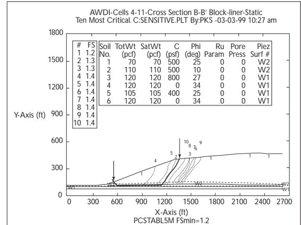
Figure 2. Slope-stability analysis.
