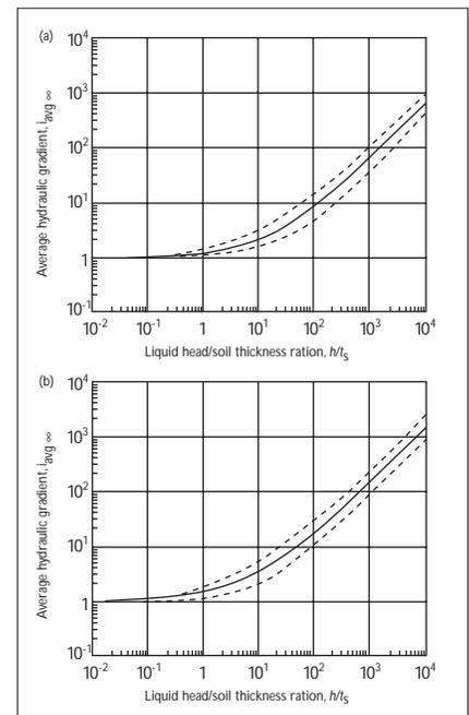
**Figure 1.** Values of the average hydraulic gradient to be used in equations for liquid migration-rate calculations: (a) with a circular or square defect, (b) with an infinitely long defect.
