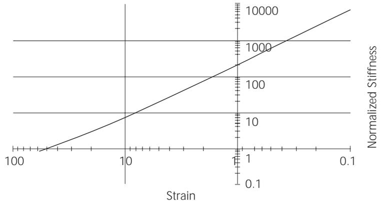
**Figure 4.** Normalized Tension Stiffness vs. Strain (Ref. Table 4 Giroud, et al. 1995).
