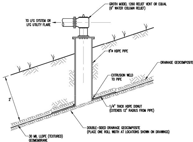
Figure 9 – Emergency Gas Relief Vent Cross Section
