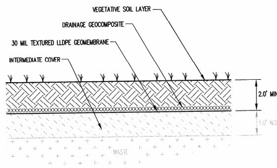
Figure 1 Typical Final Cover System
