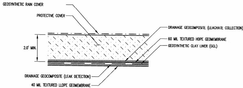
Figure 2 Typical Piggyback Liner System
