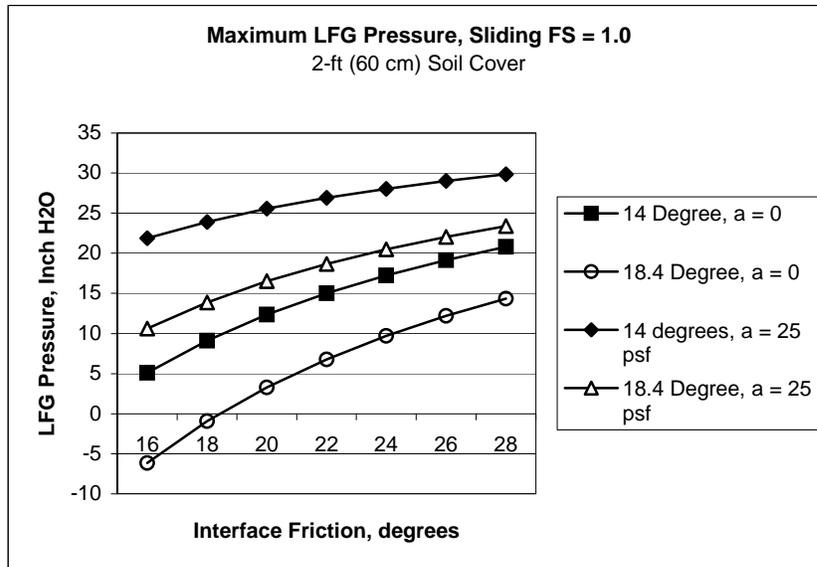
Figure 3 LFG Pressure at Limit of Sliding Stability, FS = 1.0
