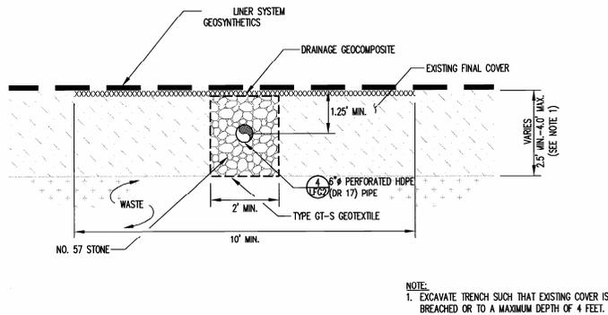
Figure 8 LFG Collector Trench Cross Section
