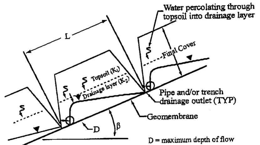
**Figure 3:** Schematic of head buildup in the drainage layer
