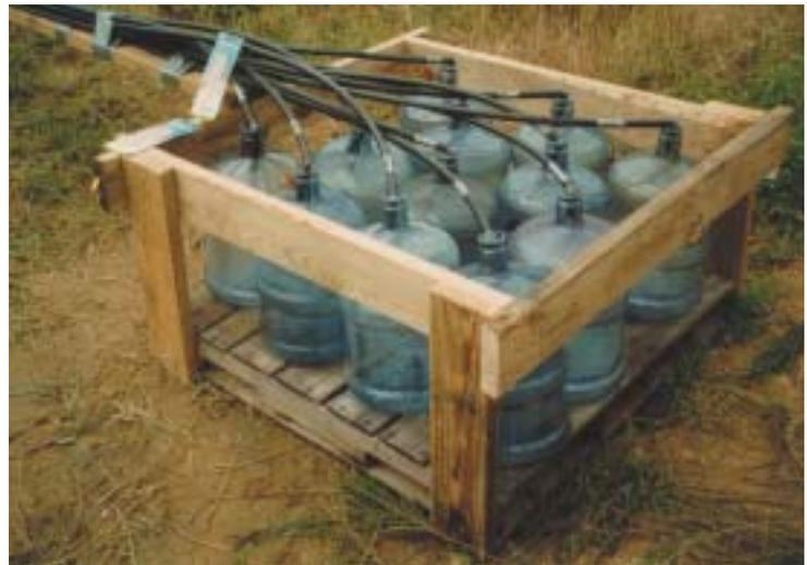
**Photo 2.** Lysimeter monitoring “sumps.”
