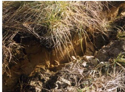
Figure 15. Cracks widening between sliding blocks
